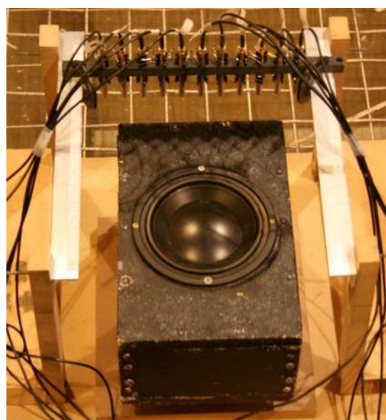
FIG. 11. (Color online) Enclosed loudspeaker source and microphone array for near-field measurement.
