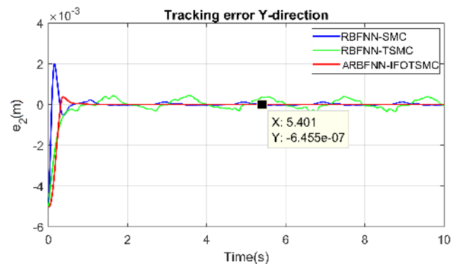
FIGURE 6. The tracking errors of the end-effector in the Y-direction.
