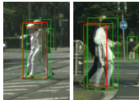
Figure 6. Failure cases of adaptive-NMS with the 0.3 visual score threshold. Red boxes are false positives. As the NMS threshold ( N_M ) increases for crowd instances, more false positives are also preserved if the proposals are not compact.
