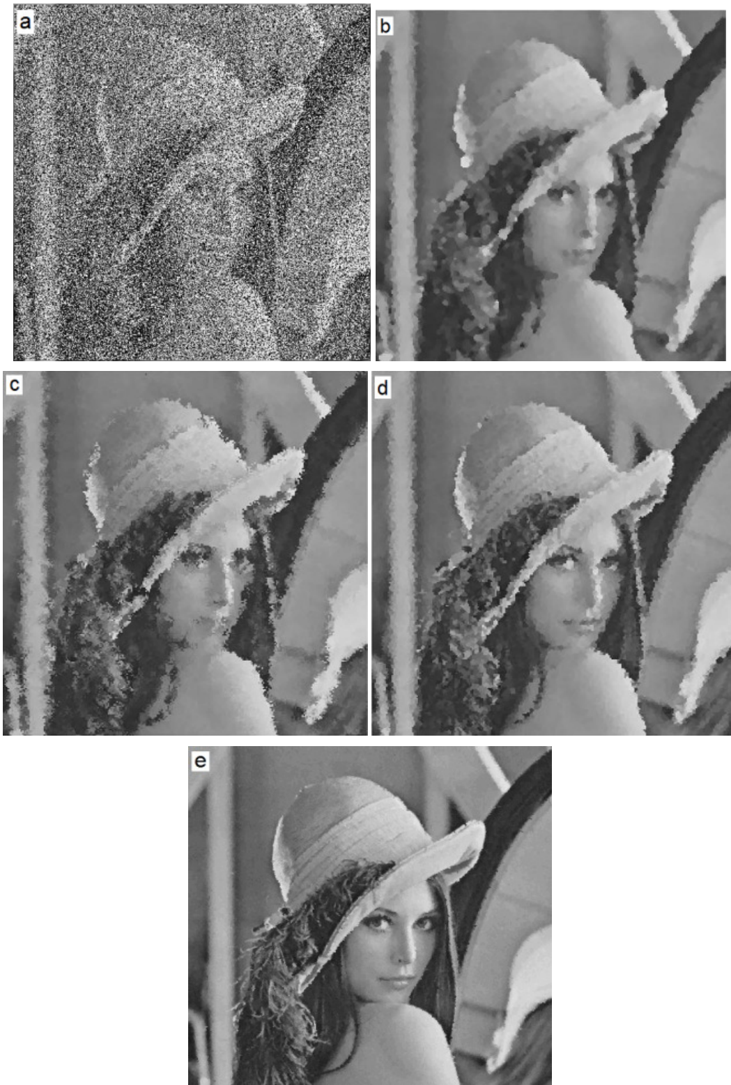
Figure 5. Image restoration results of the Lena image. (a) 80% noise corrupted, (b) DBA, (c) AMF, (d) CBA, (e) proposed
