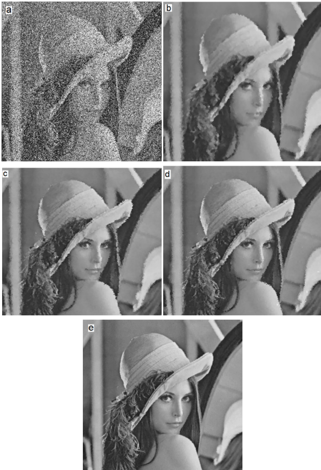
Figure 4. Image restoration results of Lena image. (a) 50% noise corrupted, (b) DBA, (c) AMF, (d) CBA, (e) proposed
