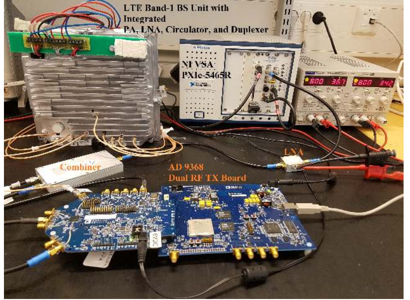
Fig. 4. The RF measurement setup used for evaluating the performance of the proposed nonlinear active RF cancellation solution: (a) block diagram of the measurement setup; (b) photo of the measurement setup.
