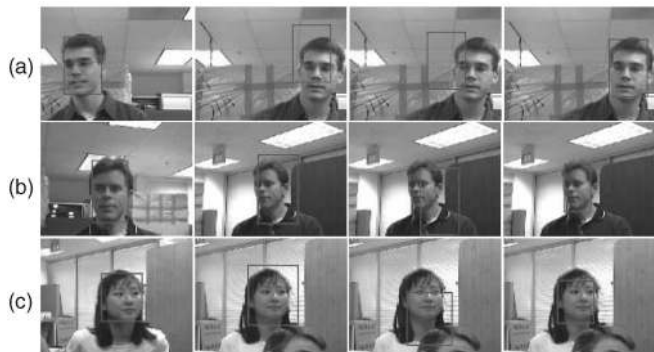
Fig. 6. Tracking results with the MS tracker (second column), the C tracker (third column), and SMOG1 (fourth column). The first column shows the initial target state. For the MS and C trackers, we use 16 \times 16 \times 16 color histogram bins. For the C and SMOG1 trackers, we use the first-order AR dynamic model [9], [20].
