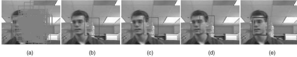
Fig. 3. An example of tracking a face with a weak dynamic model: (a) 100 particles configurations out of the 5,000 particles. (b), (c), and (d) The results using the color histogram-based similarity measure with (b) 4 \times 4 \times 4 bins, (c) 8 \times 8 \times 8 bins, and (d) 16 \times 16 \times 16 bins. (e) The results for the proposed method with k = 5 , k = 7 , and k = 9 .
