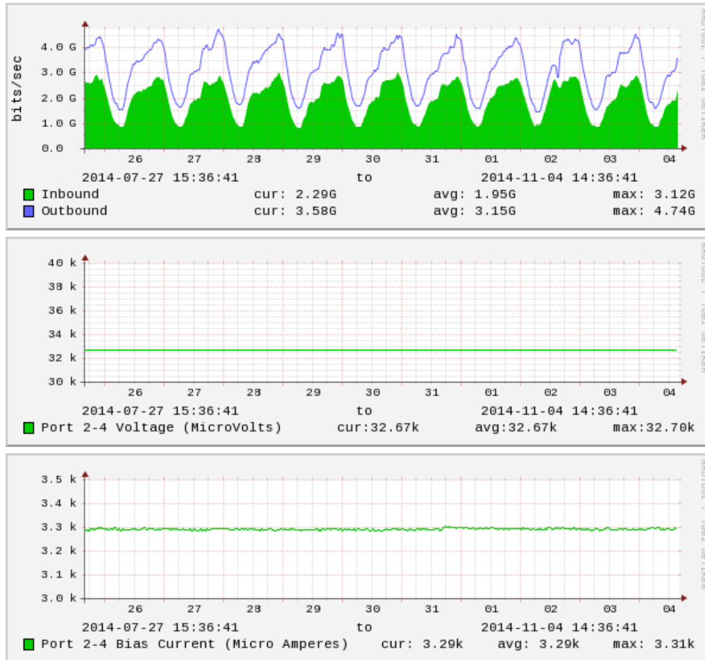
Figure 3. Traffic load (top), supply voltage (middle) and Tx bias current (bottom) of 10 Gbit/s link.
