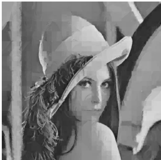
Figure 3: 512x512 Lenna compressed using Fisher's quadtree coder, compression ratio = 1:28.1, PSNR 28.8 db
