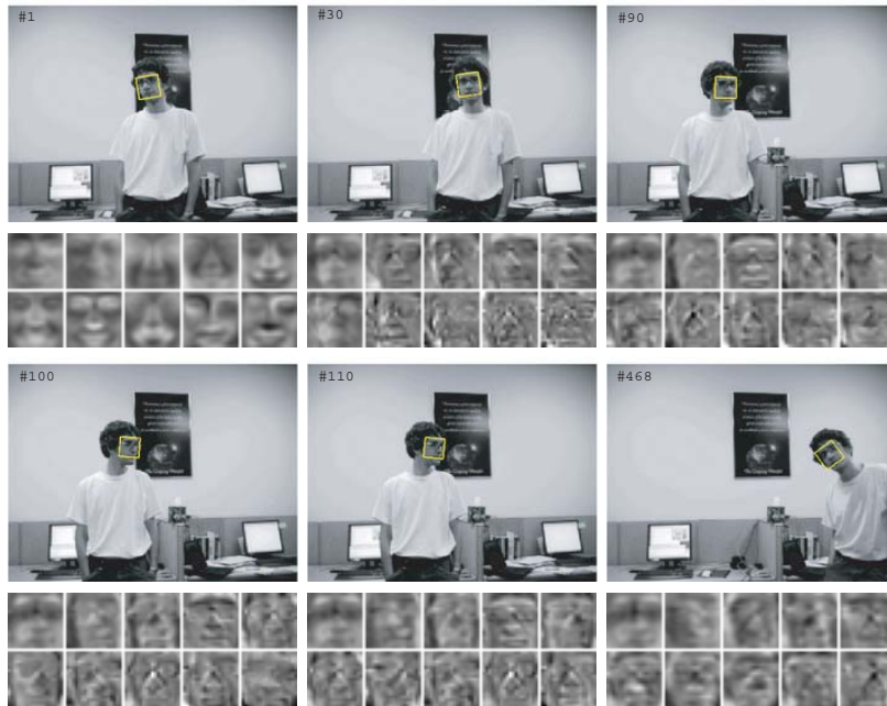
Fig. 2. Tracking an object undergoing a large pose variation (See video at http://www.cs.toronto.edu/~dross/ivt/ ).
