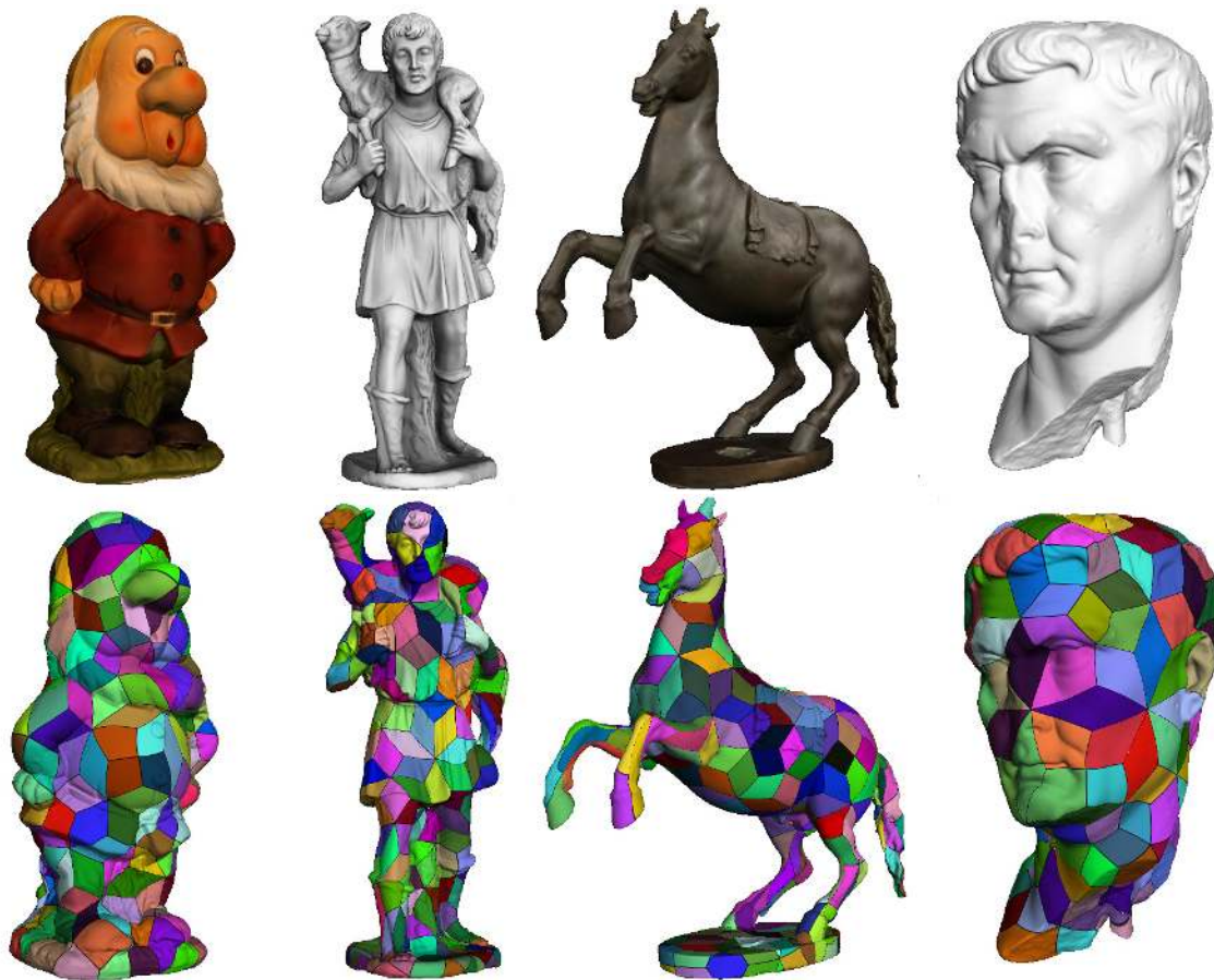
Figure 7: Models rendered with the adaptive quad patch method. Top row shows the rendered models at pixel tolerance one. Bottom row shows the patch structure. Complexity ranges from 6.4 to 62.5M samples.
