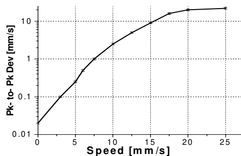
Fig. 11. Peak-to-peak OCT image surface displacement rate with AR on versus the surface velocity with AR off.
