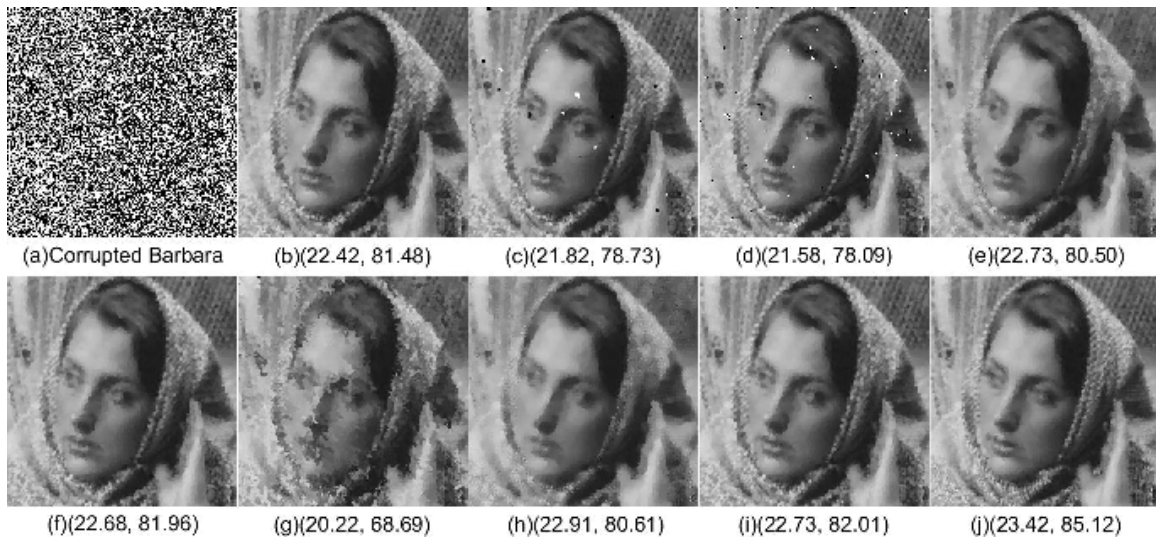
FIGURE 11. Recovery results of image Barbara with 80% impulse noises.(a) Zoomed-in local part of Barbara with impulse noise; Results of (b) DAMF; (c) NDBINF; (d) PVGF; (e) ADWMF; (f) RBF1; (g) SVMFF; (h) NAISM; (i) INLM; (j) ASWMF.
