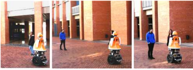
Fig. 1 Real-life experiments of the user study: Left: Tibi Robot accompanies a person in an urban environment. Center: The pair robot-human, approaches a pedestrian in the surroundings. Right: The three members share the personal space while have a conversation.
