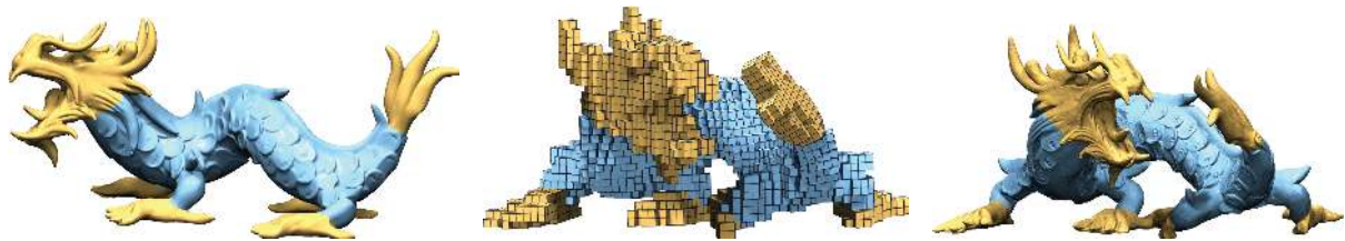
Figure 8: Deformations on a very large model. The user deforms the shape using a reduced model during interaction shown on the left. When satisfied with her results, the final space deformation is applied offline to the high-resolution model on the right consisting of more than seven million triangles.
