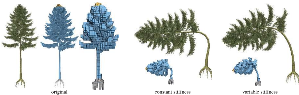
Figure 9: Deformation of a triangle soup consisting of 14k connected components. The leaves of the tree are modeled as alpha-textured triangles. On the right the stiffness was decreased toward the top of the trunk and for the leaves.
