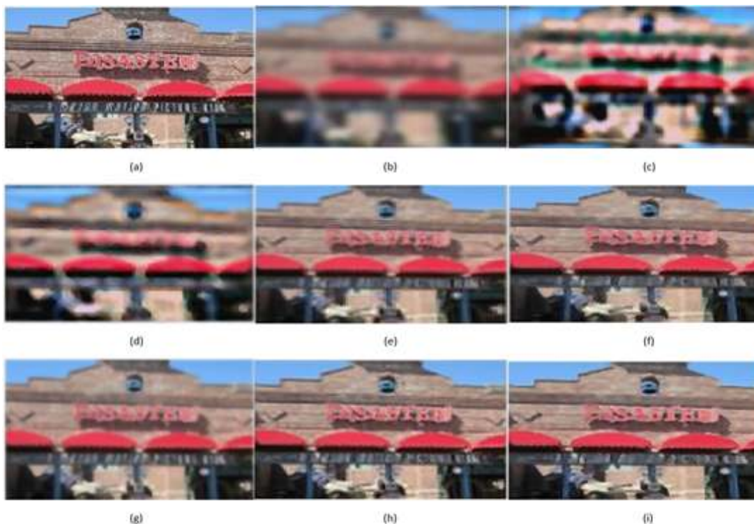
Fig 14. Comparison of image deblurring results of different methods: (a) Original Image (b) Image blurred through Uniform Blur (c) Deblurred using Sobolev Priors (d) Deblurred using TV Priors (e) Deblurred using Gaussian Priors (f) Deblurred using L1 Priors (g) Deblurred using Tikhonov Priors (h) Deblurred using Sparse Priors (i) Deblurred using the proposed method (SAP)
