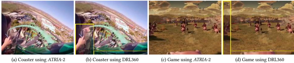
Figure 7: Frame captures of video session for two videos each with ATRIA-2 and DRL360 . Video frames at (b) and (d) show that parts of the viewport have poor image quality (yellow rectangular areas) for DRL360 .
