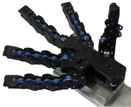
Fig. 1. THE UNIPI hand, a self-contained humanoid robotic hand powered by adaptive synergies.
