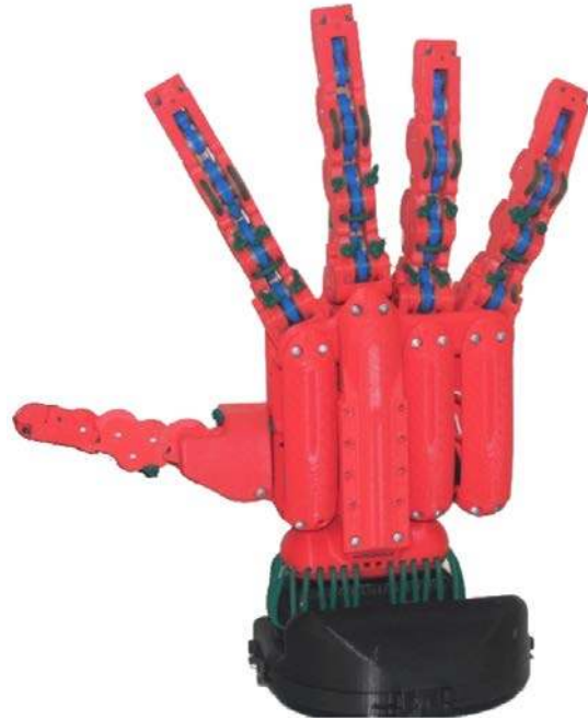
Fig. 1. Skeleton of the Pisa/IIT SoftHand advanced anthropomorphic hand prototype implementing one adaptive synergy. The prototype dimensions are comparable to those of the hand of an adult human.
