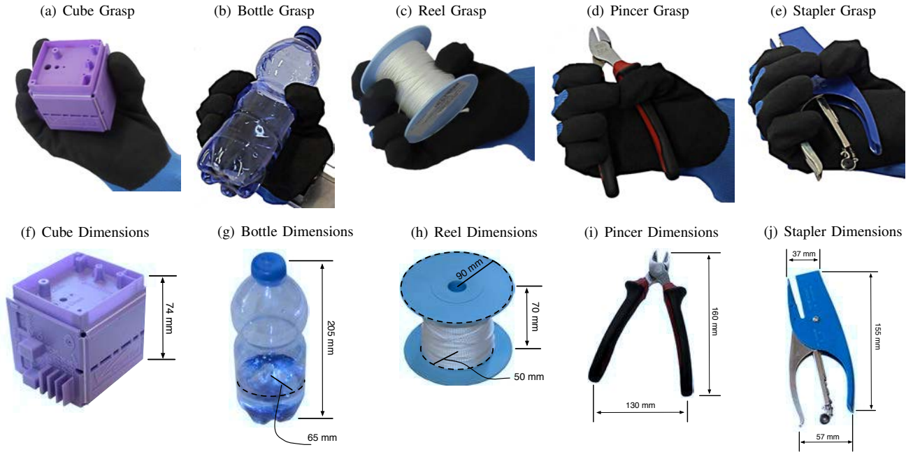
Fig. 20. Some experimental grasps performed with the Pisa/IIT hand, with the object placed in the hand by a human operator.
