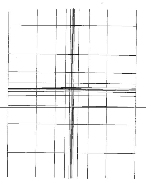
Figure 1. Example of how a tensor product grid might adapt to a point singularity in a function of two variables.
