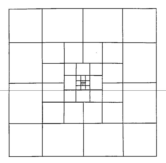
Figure 2. Example of how adaptive grid refinement might adapt to a point singularity in a function of two variables. The grid in Figure 1 is a refinement of this partition.
