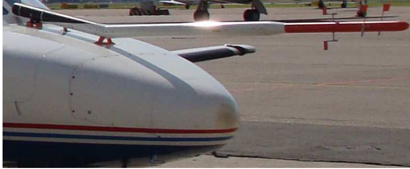
Fig. 6: The vanes on the boom for measuring the angle of attack and angle of sideslip. Photo credits by Daan Pool.
