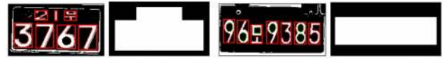
FIG. 8. Two reference images: Connected components of characters and their segmented inner area and outer area.
