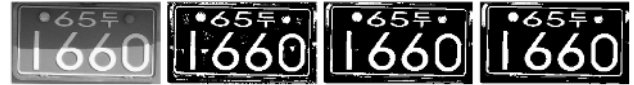
FIG. 7. Post-processing results: (a) gray image; (b) binarized result before post-processing; (c) result of post-processing by CAM_1 ; (d) result of post-processing by CAM_2 .
