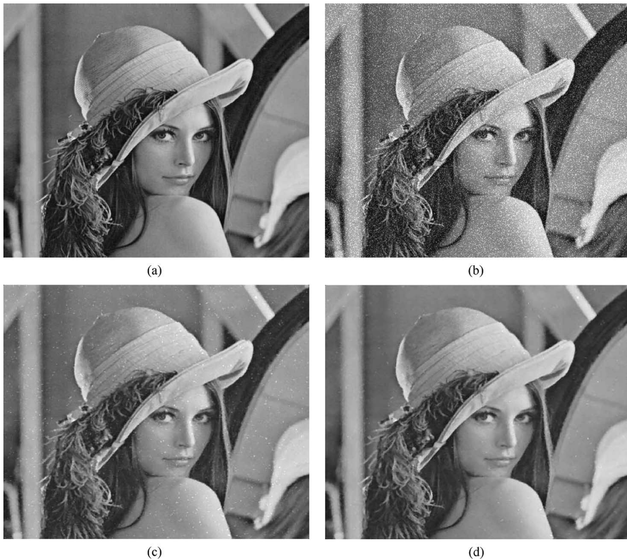
Fig. 3. Standard median filter to remove impulse noise: (a) original image; (b) noisy observation; (c) restored image by the 3 \times 3 median filter; and (d) restored image by the ATPMF. Noise ratio is 25%. Impulse noise has a Gaussian distribution with mean 30 and standard deviation of 5.
