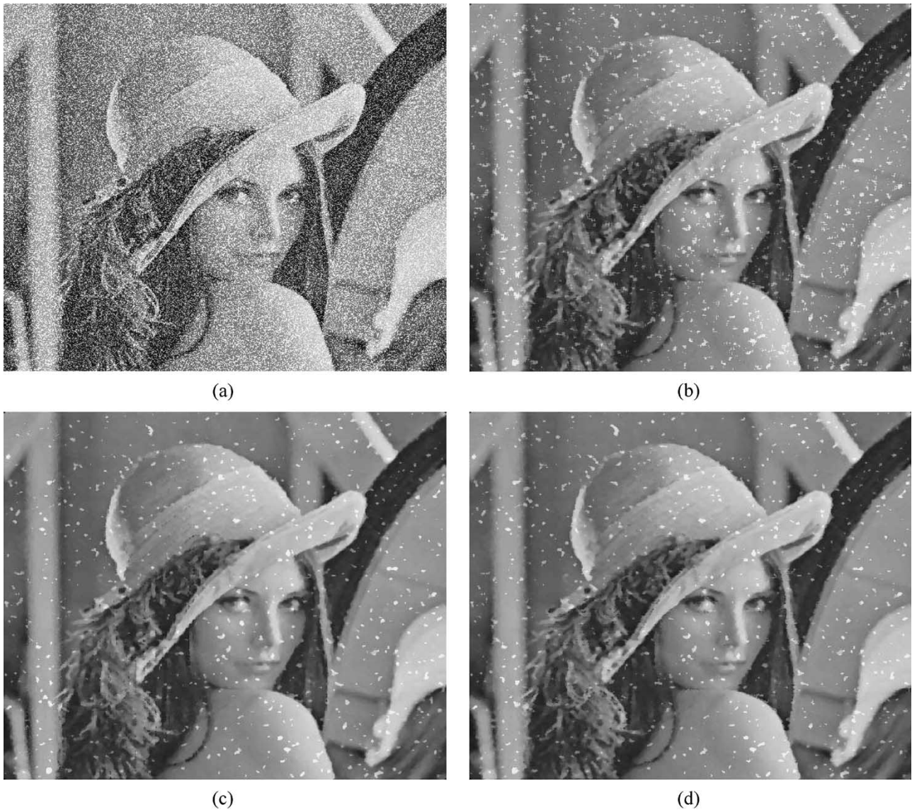
Fig. 5. Different implementation. (a) Noisy observation of “Lena,” noise ratio is 35%. (b) Restored image by a standard 5 \times 5 filter, PSNR = 20.8517 (dB). (c) Restored image by ATPMF implemented in columns, PSNR = 22.8672 (dB). (d) Restored image by ATPMF implemented in rows, PSNR = 22.7692 (dB).
