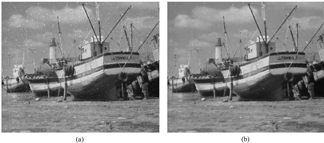
Fig. 8. Restored “boat” image by: (a) the 3 \times 3 median filter, PSNR = 25.0612 (dB) and (b) an ATPMF implemented in rows, a = 1 , b = 1 , PSNR = 27.7221 (dB). Noise ratio is 20%. Noise has a uniform distribution between 0 and 80.
