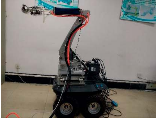
FIGURE 5: The grasping experimental platform for apple harvesting robot.
