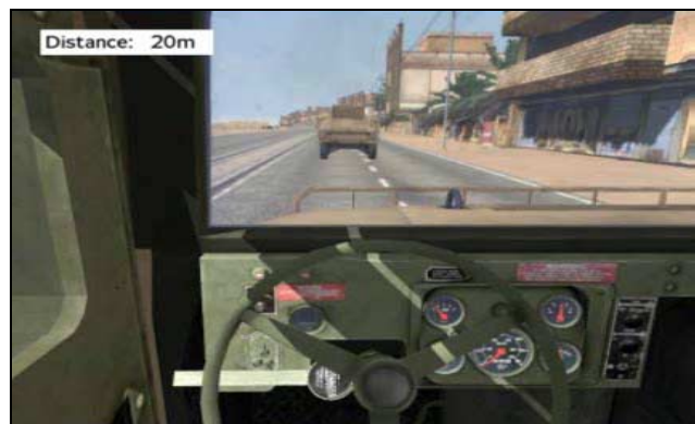
Fig. 4. Humvee following simulation. Game players are instructed to maintain their initial separation from the lead vehicle (LV) despite changes in speed of the LV. The driver's vehicle is positioned 23 meters behind the LV and s/he is instructed to maintain the distance through acceleration and deceleration.
