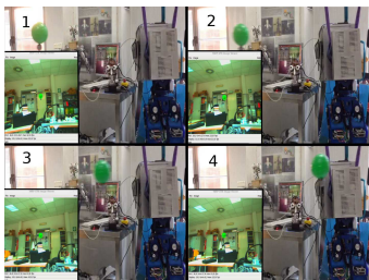
Fig. 9. Four snapshots acquired during the pursuit experiment with 0.4 Hz frequency. In big images it is shown the SABIAN head looking at the target, in small windows it is shown the left eye camera image.
