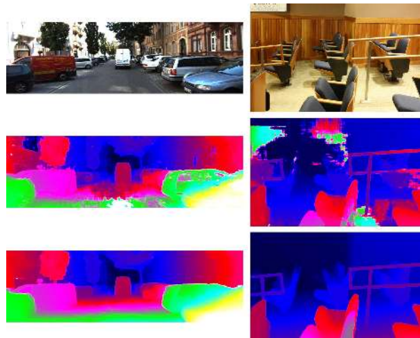
Figure 1. Overview examples. Left-right: KITTI [25] and Middlebury [30]. Top-down: left image, disparity maps predicted by the SceneFlow-pretrained PSMNet [4], and by our Ada-PSMNet.
