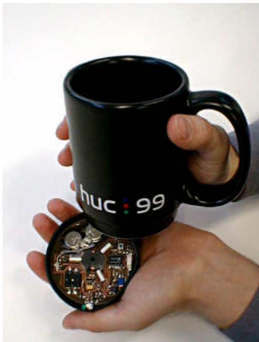
Figure 3. The Mediacup is an ordinary coffee cup with sensors, processing and communication embedded in the base.
