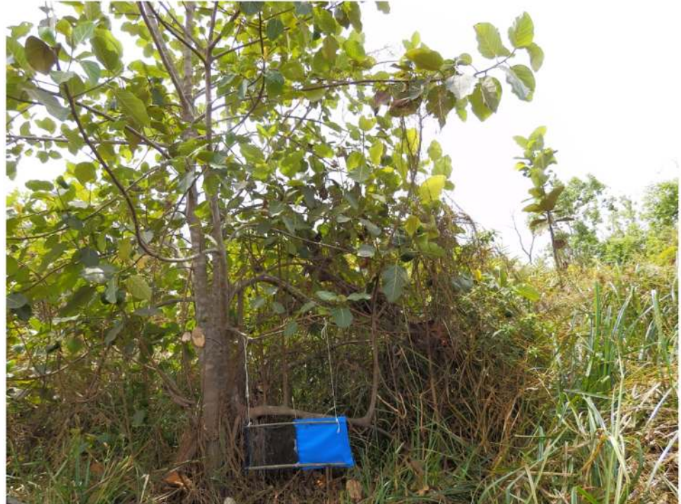
Fig 1. A tiny target suspended from a branch. Tsetse collide with the deltamethrin-treated target and pick up a lethal dose of insecticide [3, 8].
