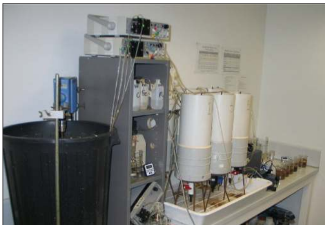
Fig. 2 Image of the porous pot experimental set up. From the left: 55 L storage container fitted with a mechanical stirrer; peristaltic pumps to transfer feedstock to the porous pots (top), additive reservoirs (centre) and peristaltic pumps to transfer additives to the porous pots (bottom); six porous pots fitted with waste taps, air tubes and heaters; air pumps.
