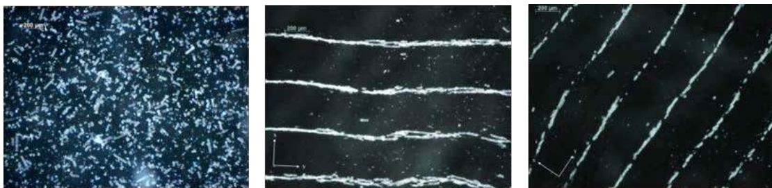
Figure 3.11: Optical Microscopy image of glass microfibre solution; (a) Randomly oriented with no acoustic field applied, (b) aligned with single 2MHz frequency, (c) aligned with frequency modulating between 2MHz and 6MHz at a frequency of 10Hz
