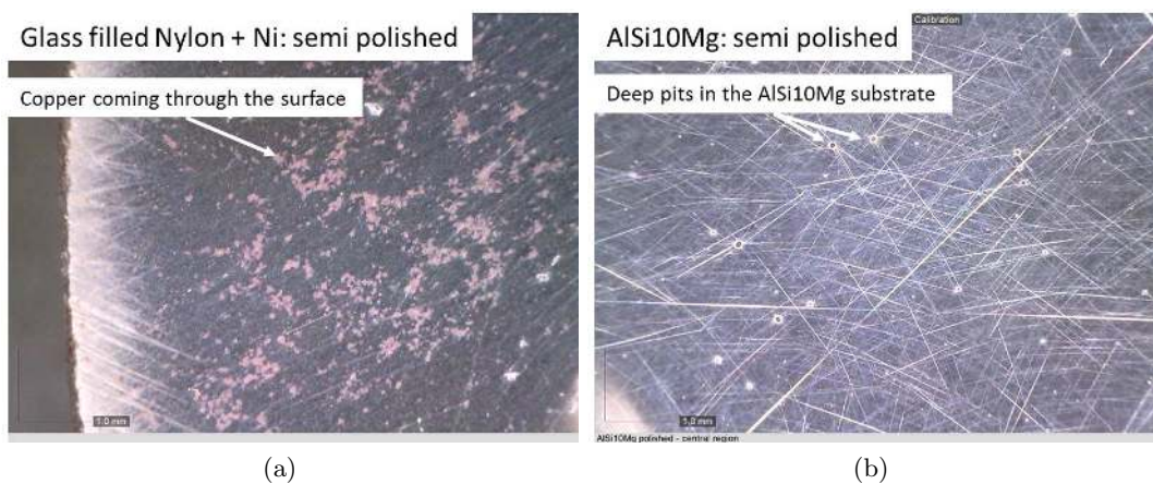
Figure 7. Microscope images highlighting the surface defects observed on the glass filled nylon sample (7(a)) and aluminium sample (7(b))
