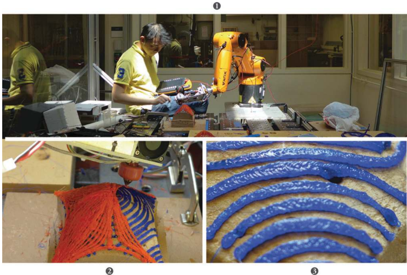
FIG. 12. Robotic fabrication work-cell setup. Photographic documentation of the robotic-enabled stress line additive manufacturing process: (1) robotic work cell; (2) oriented filament deposition of stress lines on substrate built from medium-density fiberboard; and (3) close-up detail of extruded filament.
