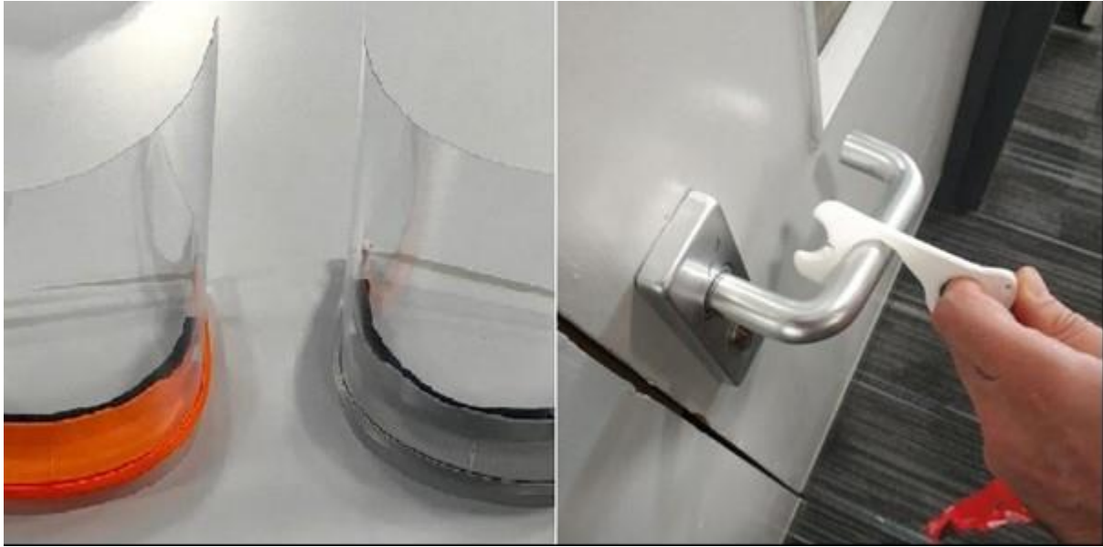
FIG. 2. Examples of 3D printed face shield and door openers prepared by the School of Pharmacy Queen’s University Belfast, donated to healthcare professionals. The face shields were made of a 3D printed part (grey/orange part), an acetate sheet as visor, an elastic band and foam to protect the forehead. These designs were approved by the infection control unit of the Belfast Health & Social Care Trust.
