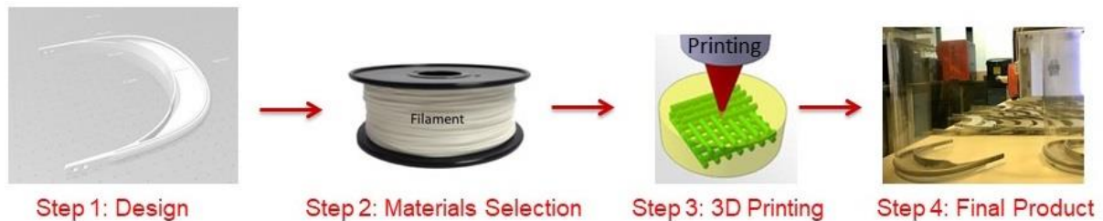
FIG. 1 Fused deposition modeling 3DP process of a face shield.
