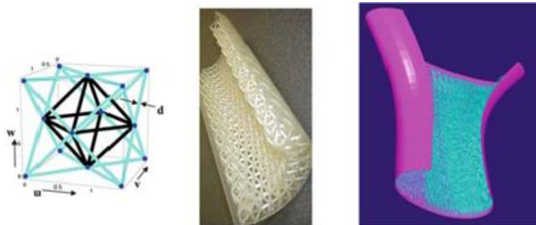
Fig. 3 Octet-truss unit cell and example parts with octet-truss meso-structures[34]
