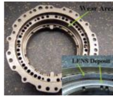
Fig. 5 Low-wattage repair of Ti-6AL-4V bearing housing [36]
