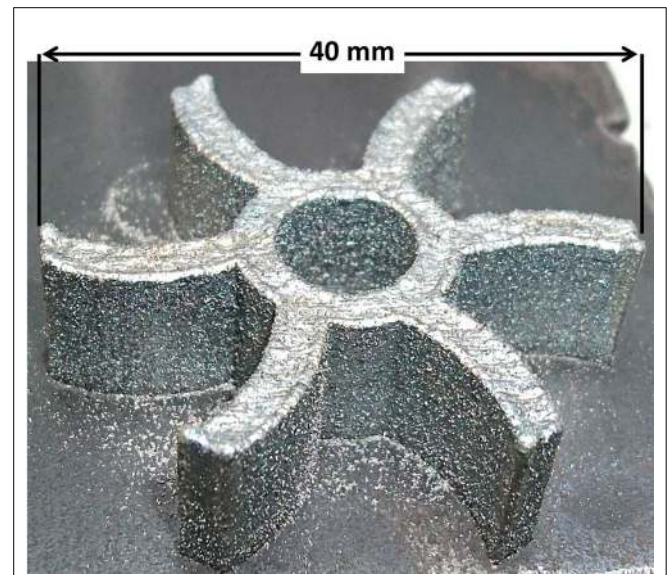
FIGURE 1 | Additively manufactured Co-Cr-Mo alloy impeller using Laser Engineered Net Shaping (LENS™).
