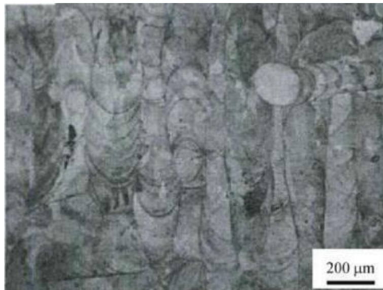
Figure 2.30 - MPBs on the cross section parallel to the laser scanning direction [82]
