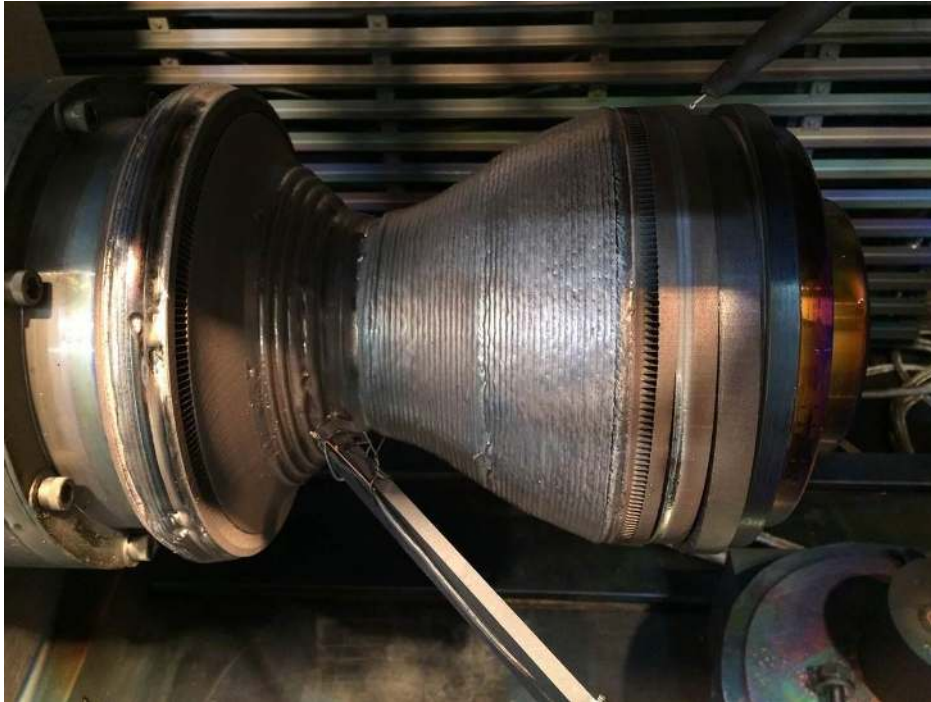
Figure 24. Development LCUSP Unit Between EBF 3 Deposition Steps.
