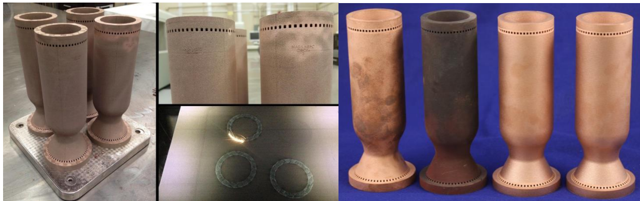
Figure 21. GRCop-84 Liners post-SLM (Left) and C-18150 Liners Post-SLM and Heat Treatment (Right), 2nd from left not grit blasted.
