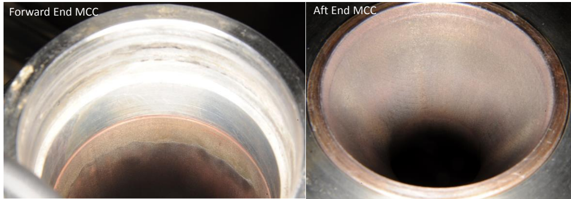
Figure 20. 3D Printed GRCop-84 Combustion Chamber liner with 2365 seconds accumulated.
