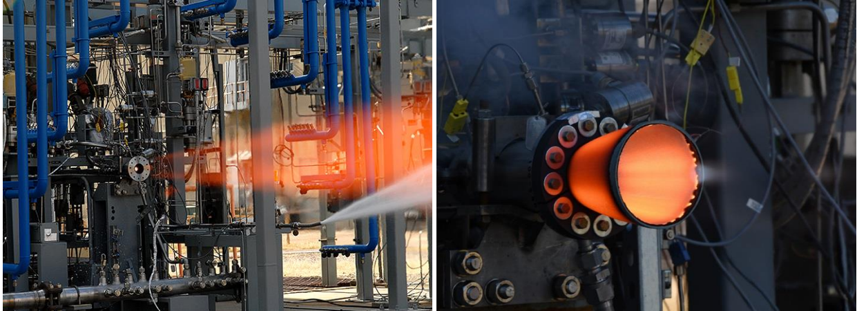
Figure 22. Hot-fire test of GRCop-84 chamber (Left) and, Hot-fire test of C-18150 Chamber Liner with OATK Carbon-Carbon Extension (Right).
