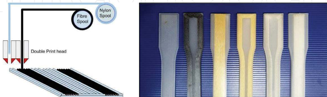
Figure 9. Schematic description of the process (left) and produced specimens with different types of reinforcement fibers (right) [21].
