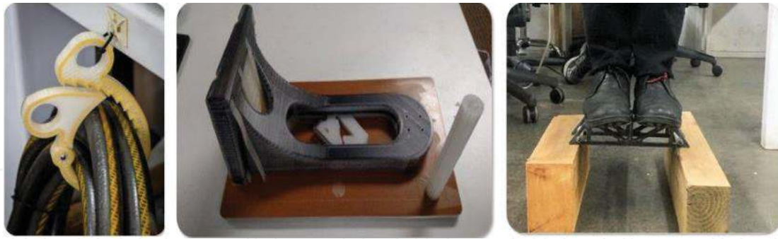
Figure 13. Holder with Kevlar reinforcement (left), head support for go-cart cars with carbon reinforcement (middle), and a structural part made of nylon and carbon fiber (right) [28].
