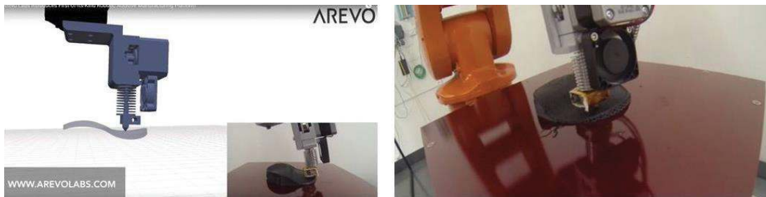
Figure 19. Six-axis composite part additive manufacturing platform from Arevo Labs [39].
