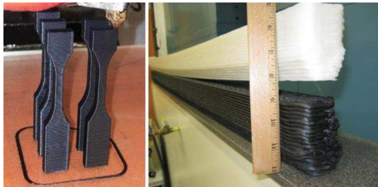
Figure 4. Tensile test specimens produced along z-axis and deformation coupons showing the difference between carbon fiber-reinforced ABS and no reinforcement part in terms of deformation [12].
