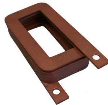
Fig. 1. Example of a shaped profile copper winding manufactured using Direct Metal Laser Sintering for a filter inductor application, [19].
