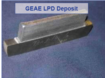
Representative feature geometries (above) and actual LPD (below left) and EBWD (below right) Nickel deposits.
