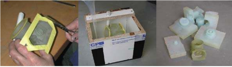
Fig. 16.13 RTV molding process steps (Courtesy MTT Technologies Group)
