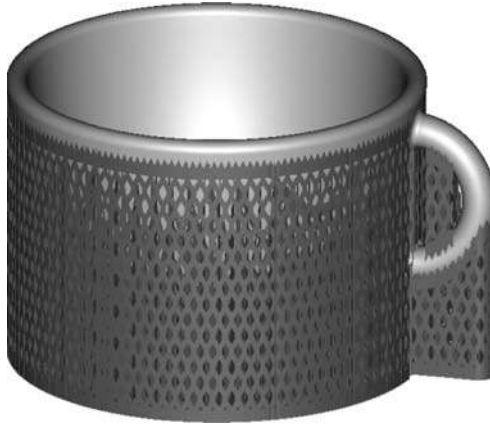
Fig. 13.4 Supports generated for a part build
