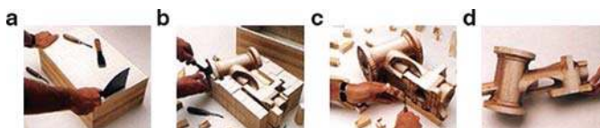
Fig. 16.2 LOM support removal process (de-cubing) process, showing: (a) the finished block of material; (b) removal of cubes far from the part; (c) removal of cubes directly adjacent to the part; (d) the finished product (Courtesy Worldwide Guide to Rapid Prototyping web-site (C) Copyright Castle Island Co., All rights reserved. Photo provided by Cubic Technologies.)
