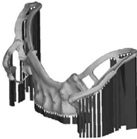
Fig. 16.5 SLM dental framework (© Emerald Group Publishing Limited) [1]
