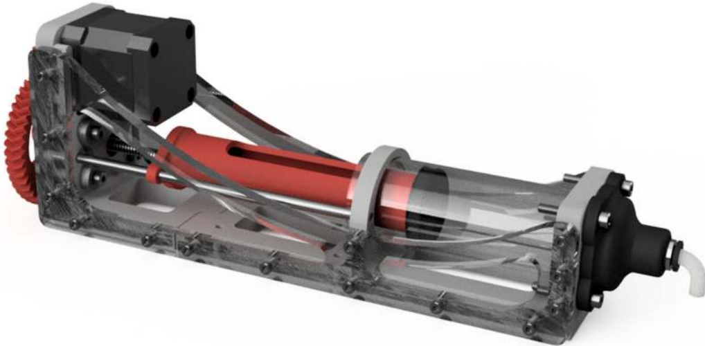
Fig. 3 The feed system was designed and rendered in Fusion 360. This feed system unit has a capacity of 100 mL, provides excellent positional precision using a geared down leadscrew, and can generate pressures over 100 psi.
