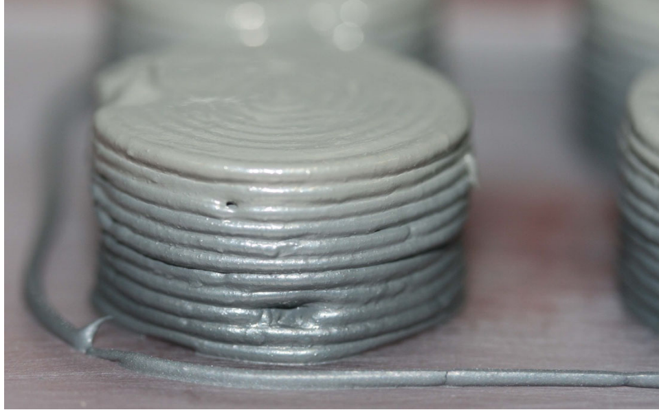
Fig. 12 Gradient boron carbide (bottom) to silicon carbide (top) 1-inch diameter cylinder produced by DIW. Print parameters are 1.2-mm layer height, 1.2-mm nozzle width, 4-mm/s print head speed, and center-to-perimeter concentric fill pattern.
