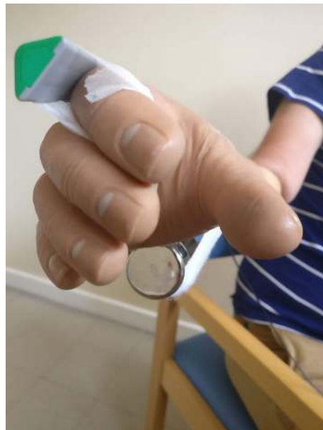
Figure 3. 500 g Load added to prosthetic hand. The load was bandaged to the hand at the proximal palm/distal wrist level so as not to disrupt the opening/closing of the hand.
