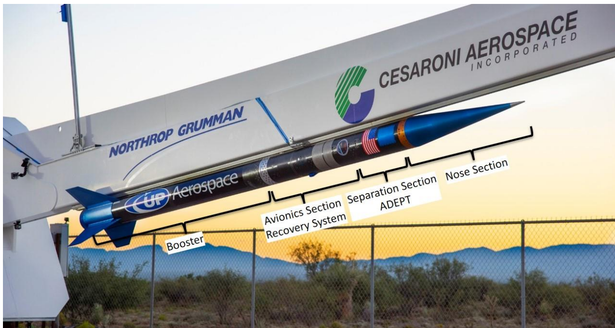
Figure 9- LV moving to launch position. ADEPT SR-1 is housed just behind the nose in the separation section.
