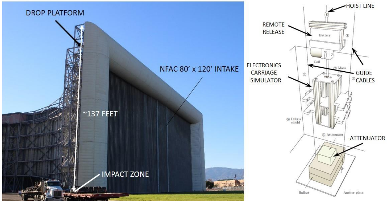
Figure 6- Impact test location and test set-up description.
