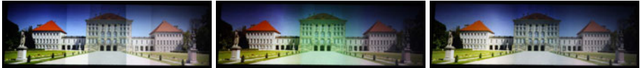
Fig. 7. Color uniformity on a display made of 3 heterogeneous projectors (LCD, LCoS and DLP from left to right): Before any color matching (left), after color matching using ideal devices method (middle) and our method (right). Note that the method for ideal devices introduces a color mismatch in the middle projector by changing the color temperature. Our method balances the brightness better, making the left projector of comparable brightness as the other two. Please zoom-in to see the differences.
