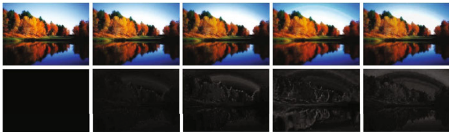
Fig. 10. Comparison of printer-to-projector color matching for a natural image. Difference from input image is shown in the second row of images. From left to right are the printed image, our method, method for ideal devices, WCS, and Adobe CMM. Note the banding artifact and less vibrancy in color due to inaccurate color match in WCS, Adobe CMM and the method for ideal devices when compared to our method. Please zoom in to see the differences.
