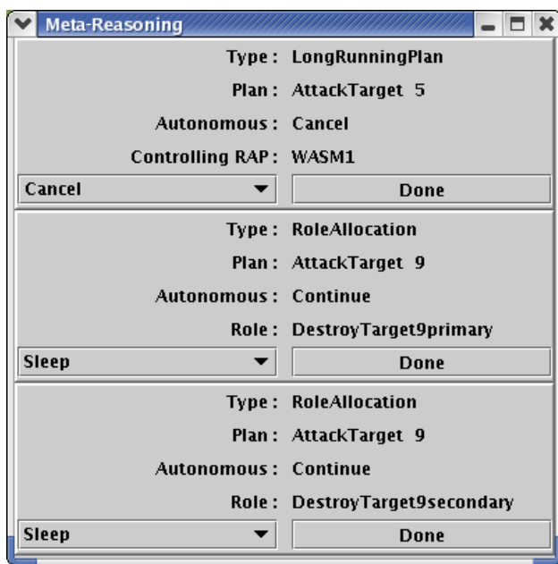
Figure 3. A view of the interface the human uses to make decisions. Three decisions are shown. At the top is a decision whether to cancel a long running plan. Below are two unallocated roles from the same plan, for destroying a particular target.
