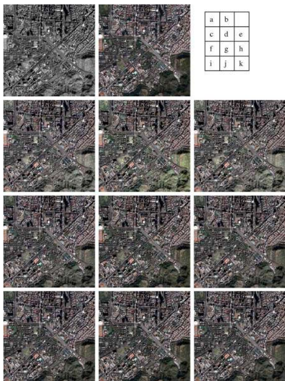
Fig. 4 A subsection of Taipei, Taiwan: (a) the output 8-bit Pan image by applying step 2 part 1; and (b) the output 8-bit RGB image by applying step 2 part 1. The fused images by (c) IHS, (d) BT, (e) IHS-BT, (f) GIHS, (g) GBT, (h) GIHS-BT, (i) SA-IHS, (j) SA-BT, and (k) SA-IHS-BT.
