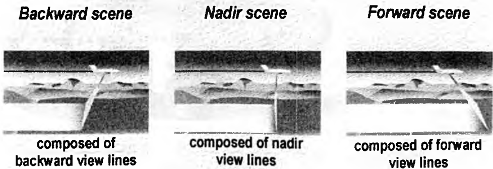
Figure 4. Three-line scanner principle
