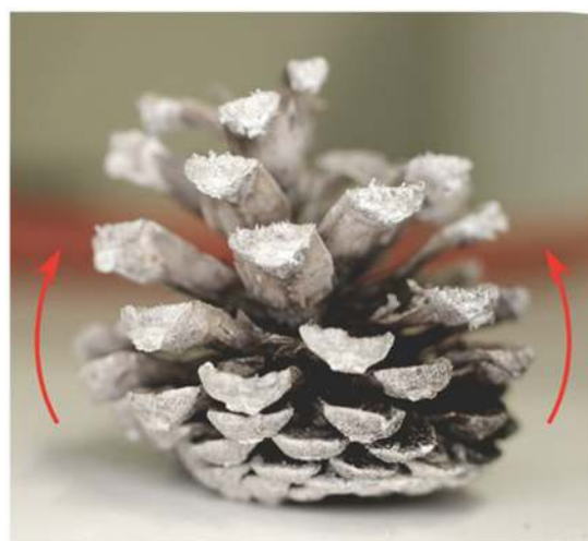
FIG. 25. An artificial pine cone made of mesoporous silica is able to mimic the behavior of its natural prototype: adsorption-induced deformation makes the ovuliferous scales of the cone move with the change of humidity. Reprinted with permission from Van Opendenbosch et al. , Adv. Mater. 28 , 5235–5240 (2016). Copyright 2016 Wiley.
