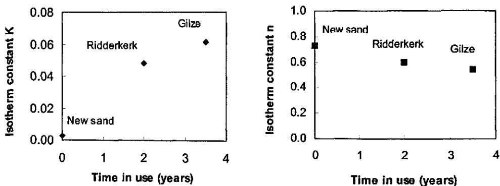
Fig. 2.3 Change in isotherm constants K and n of filter media with time in use
